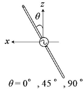
Fig. 7. Polarization directions of the receiving antennas.
