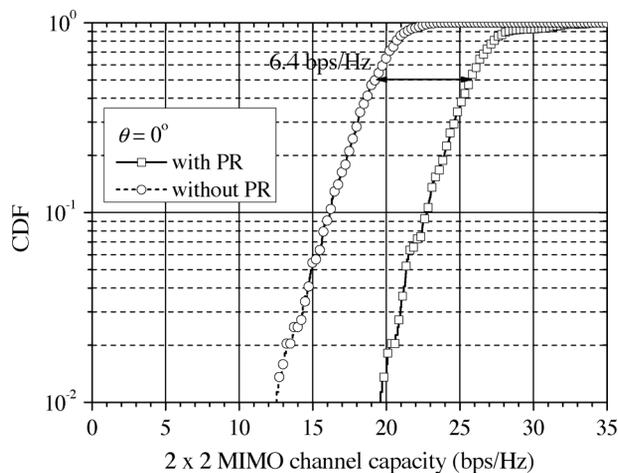
Fig. 9. CDF of the  $2 \times 2$  MIMO channel capacity with/without four-unit PR for vertical polarization ( $\theta = 0^\circ$ ).
