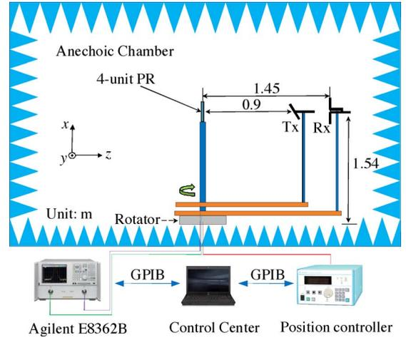
Fig. 3. Measurement system in the anechoic chamber.
