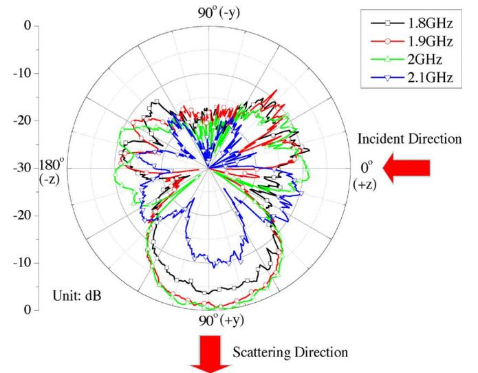
Fig. 4. Normalized BRCS of the four-unit PR at various frequencies.
