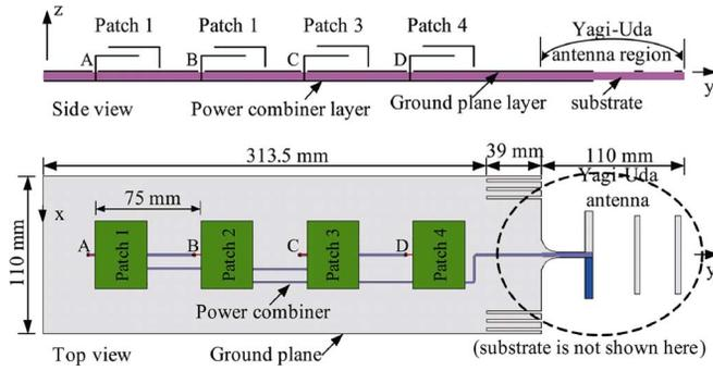
Fig. 1. Configuration of one-unit PR.
