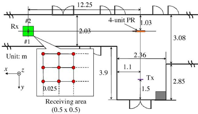
Fig. 5. MIMO measurement environment.
