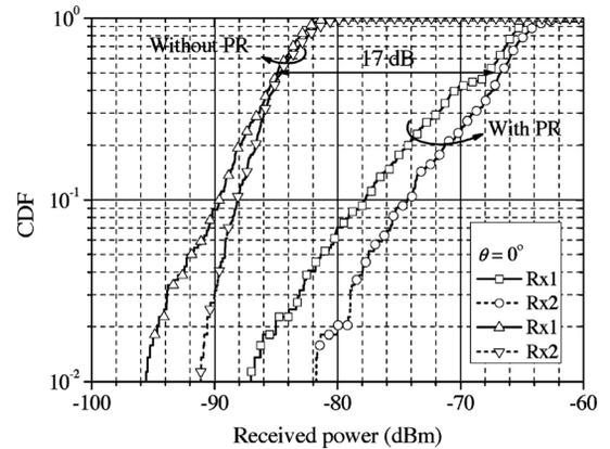
Fig. 8. CDF of the received power with/without four-unit PR for vertical polarization ( $\theta = 0^\circ$ ).
