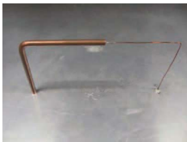
Figure 11 Fabricated loop antenna2 with different radius. [Color figure can be viewed in the online issue, which is available at wileyonlinelibrary.com ]
