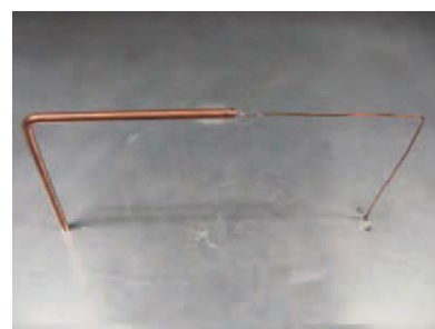
Figure 9 Fabricated loop antenna1 with different radius. [Color figure can be viewed in the online issue, which is available at wileyonlinelibrary.com ]
