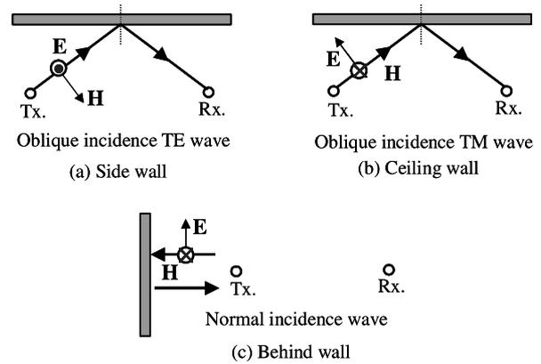
Fig. 2 Calculation model of wall reflection coefficient.
