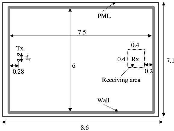
Fig. 1 Plan view of indoor MIMO analysis model (Unit: m).
