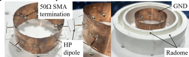
Fig. 7. Fabrication of the proposed antenna.
