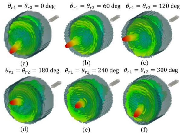
Fig. 7. The simulated 3-D radiation patterns of reconfigurable prism concept operating at 30GHz by rotating two phase plates along the same direction with the same angle (a)  $\theta_{r1} = \theta_{r2} = 0^\circ$ . (b)  $\theta_{r1} = \theta_{r2} = 60^\circ$ . (c)  $\theta_{r1} = \theta_{r2} = 120^\circ$ . (d)  $\theta_{r1} = \theta_{r2} = 180^\circ$ . (e)  $\theta_{r1} = \theta_{r2} = 240^\circ$ . (f)  $\theta_{r1} = \theta_{r2} = 300^\circ$ .
