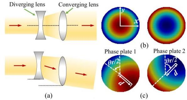
Fig. 3. (a) The beam deflection in a specific direction like a prism using Galilean afocal lens pair system with opposite optical powers. (b) Schematic of phase distribution for the lens pair with opposite optical powers. Left: diverging lens; Right: converging lens. (c) Schematic of the corresponding decentered phase distribution.
