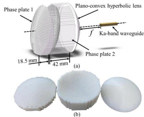
Fig. 5. (a) Schematic of experimental setup for verification of reconfigurable prism concept. (b) The prototype of the proposed decentered phase plate and plano-convex hyperbolic lens with PLA plastic material.
