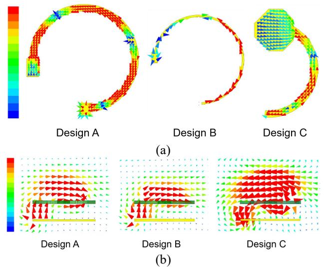
**Figure 2.** Comparisons of the electric current and field distributions of the Design A, Design B and Design C (proposed). (a) Electric currents distributions on semi-annular microstrip with hexagonal patch. (b) Electric field distribution in near zone.
