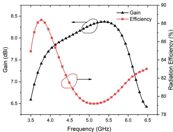
**Figure 4.** Simulated gain and radiation efficiency of the proposed PADA.
