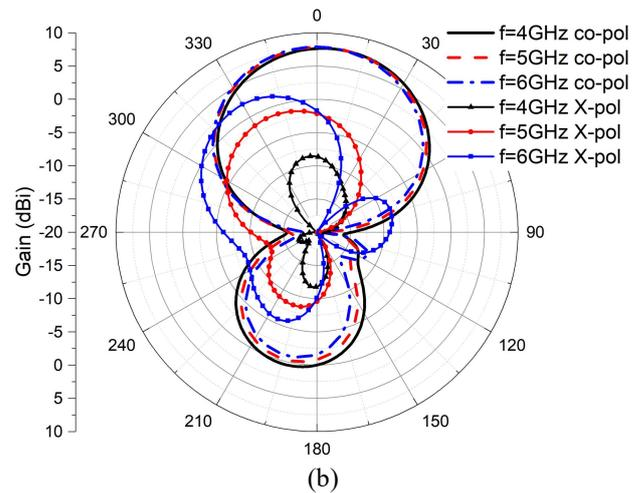
**Figure 5.** Radiation patterns of the proposed PADA in the operation frequency band. (a) E plane. (b) H Plane.
