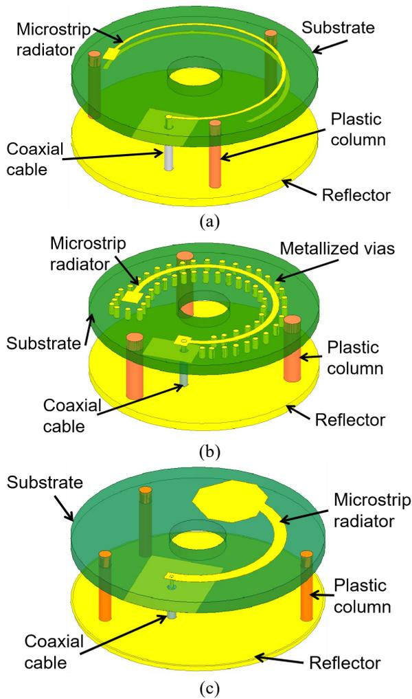
**Figure 1.** Geometries of partial-annular directional antennas. (a) Design A. (b) Design B. (c) Design C (proposed).
