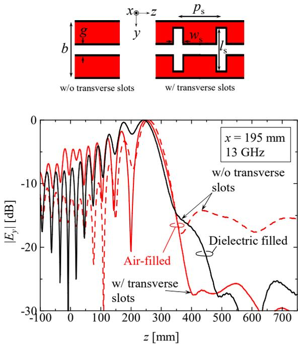
**Fig. 3.** Normalized radiated electric field from air-filled and dielectric-filled waveguide LWA models extracted from full-wave simulation.
