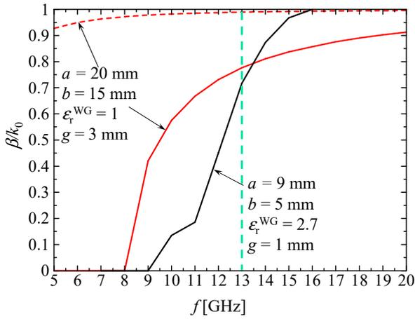
**Fig. 2.** Normalized phase constant in air-filled ( $\epsilon_r^{\text{WG}} = 1$ ) and dielectric-filled ( $\epsilon_r^{\text{WG}} = 2.7$ ) waveguide LWAs.
