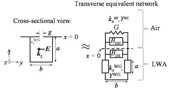
Fig. 1. Transverse equivalent network of the uniform rectangular waveguide leaky-wave antenna.
