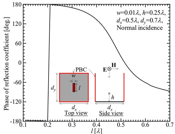
Fig. 1. Reflection coefficient of planar dipole element backed by ground plane.
