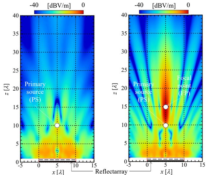
Fig. 3. Near-field distribution of designed reflectarrays (Left: Reflectarrays focusing on broadside direction in far-field region, Right: Reflectarrays focusing on a specific focal point,  $y = 7\lambda$ ,  $E_y$  components).
