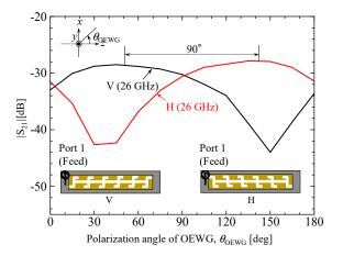
Fig. 4. Measured transmission coefficient between between OEWG and LWFA for different polarization angles of OEWG  $\theta_{\text{DEWG}}$ .
