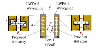
Fig. 1. Previous and proposed slot array antenna structures.
