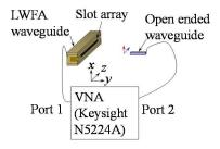
Fig. 2. Experiment setup to measure radiated component of electric field.
