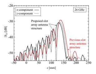
Fig. 3. Measured transmission coefficient between OEWG and LWFA with previous and proposed slot array antenna structure.
