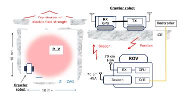
Fig. 15. An idea how to make a field strength map by the crawler robot and how to find a position of the underwater robot.
