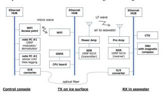
Fig. 10. Function blockdiagram of the function model for communication test
