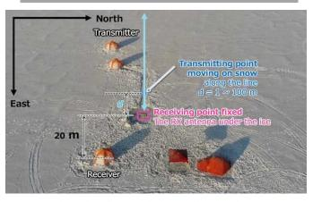
Fig. 4. Experimental configuration for horizontal propagation measurements in Saroma lake. Upper: cross-section view and lower: a snap shot of the test site in 2020.
