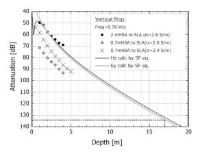
Fig. 9. An air-ice-sea boundary propagation in vertical at 10 kHz.
