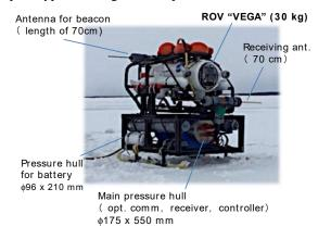
Fig. 13. The ROV equipped with the beacon, the antennas, and the pressure hulls.
