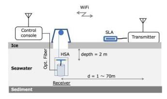
Fig. 12. Field set up of communication tests.
