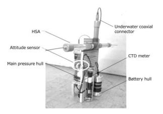
Fig. 11. An extorior view of the underwater receiver unit (RX). The 2 m-HSA is mounted on the top side of the frame. Its hight is about 0.7 m and weight is about 20 kgs.
