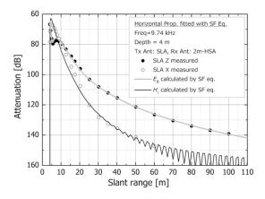
Fig. 8. Low frequency attenuation measured between air, sea-ice, and seawater in Saroma lake.at 10 kHz.
