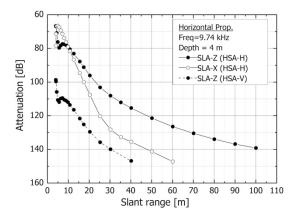
Fig. 6. Attenuation measured between air, sea-ice, and seawater in Saroma lake at frequency of 10 kHz.
