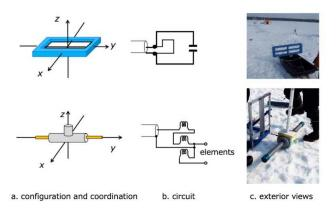
Fig. 3. Antennas developed for the experiments. Upper: SLA and Lower: HSA. Upper right picture shows the SLA on a sled. Lower right picture shows the 2 m HSA with a 5 m FRP rod.
