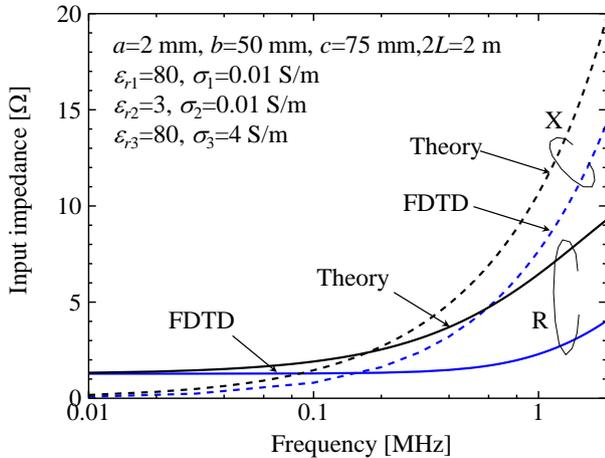
Fig. 2 Input impedance of half sheath dipole antenna with PVC-cover in seawater.
