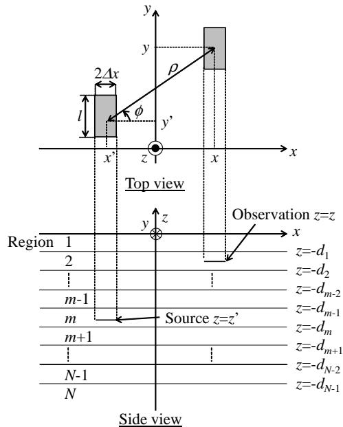
Fig. 1. Two planar microstrip segments in a thin-stratified medium.
