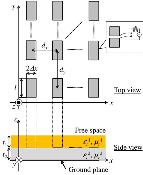
Fig. 2. Microstrip dipole array antenna embedded in a double layered medium backed by a ground plane.
