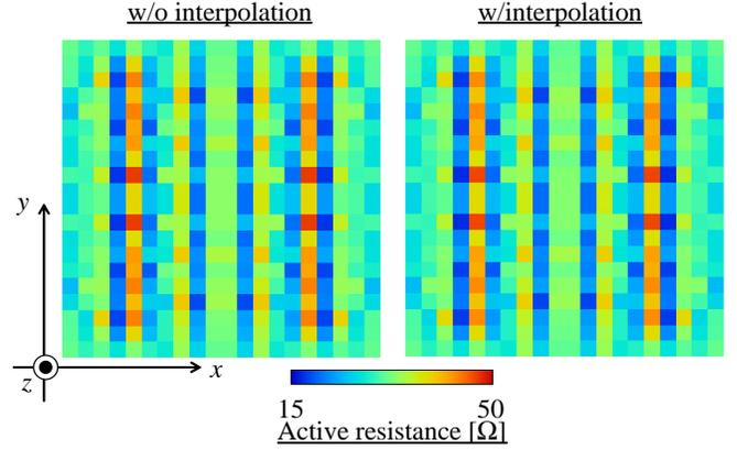
Fig. 3. Active resistance of a  $20 \times 20$  array of microstrip dipole antennas ( $f = 20$  GHz,  $l = 5$  mm,  $2\Delta x = 1$  mm,  $t_1 = 2$  mm,  $t_2 = 1$  mm,  $d_x = d_y = 7$  mm,  $\epsilon_r^1 = 2.6$ ,  $\mu_r^1 = 1$ ,  $\epsilon_r^2 = 2.15$ ,  $\mu_r^2 = 1$ ).
