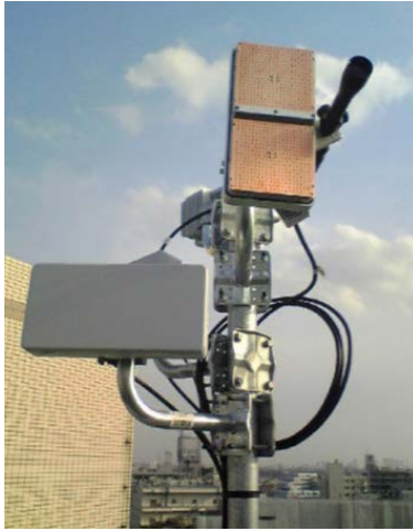
Fig. 6 A 38GHz compact one-box type wireless terminal which accommodates Tx and Rx array antennas.
