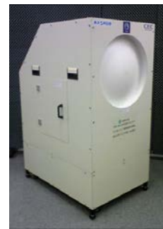
Fig. 5 Photograph of 77 GHz millimeter wave passive imaging system developed by Tohoku University, Maspro Denkoh Corp. and Chuo Electronics Co., Ltd. [33]
