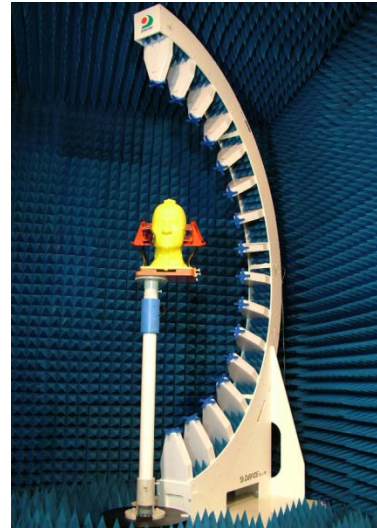
Fig. 2 A fast 3-D radiation pattern measurement equipment using parallel modulated probe array.
