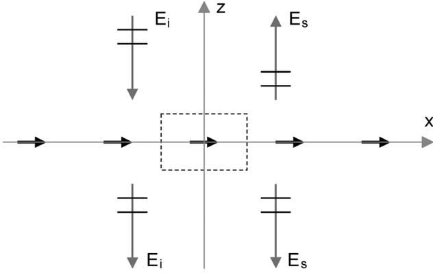
Fig. 1. Geometry of an infinite dipole array in free-space excited by a plane wave. The dipole array extends infinitely far in the  $x$  and  $y$  directions, and has dissipative loads (not shown).
