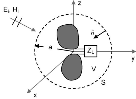
Fig. 3. An arbitrary 3D antenna of finite dimensions subject to the incident field  $\bar{E}_i, \bar{H}_i$ . The antenna is enclosed within a sphere of radius  $a$ .
