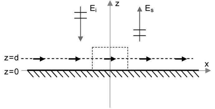
Fig. 2. Geometry of an infinite dipole array over a perfectly conducting ground plane. The dipole array extends infinitely far in the  $x$  and  $y$  directions, and has dissipative loads (not shown).
