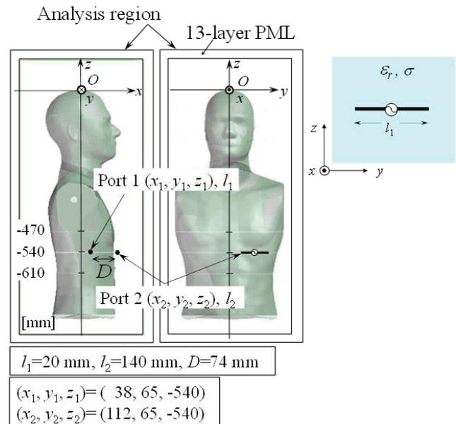
Figure 1: Human torso-shaped model with dipole antennas.
