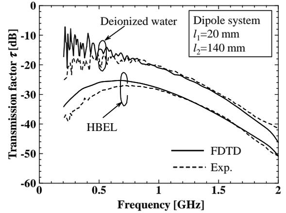
Figure 4: Transmission factor  $\tau$  of dipole antennas through torso-shaped phantom.
