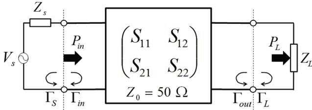
Figure 3: Two-port equivalent circuit.
