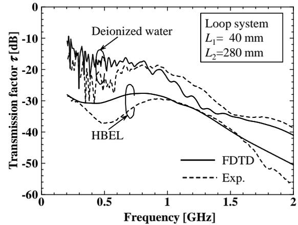
Figure 6: Transmission factor  $\tau$  of loop antennas through torso-shaped phantom.
