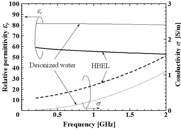
Figure 2: Relative permittivity and conductivity of deionized water and HBEL.
