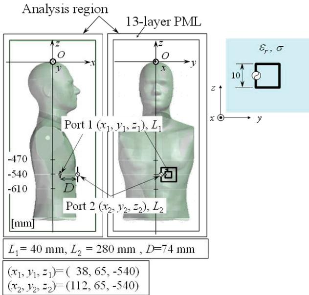
Figure 5: Human torso-shaped model with loop antennas.
