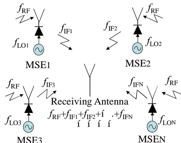
Figure 1. Configuration of MSAA
