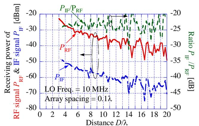
Figure 5. Receiving power versus distance  $D$
