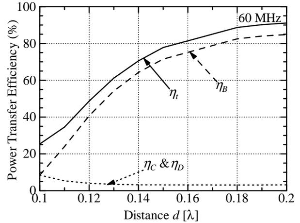
Fig 8: Frequency characteristic of PTEs when change  $d$
