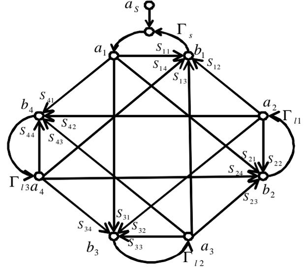
Fig 2: Signal flow graph of 4-port network
