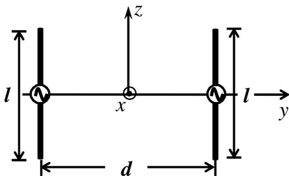
Fig 4: 2-port WPT system for comparison
