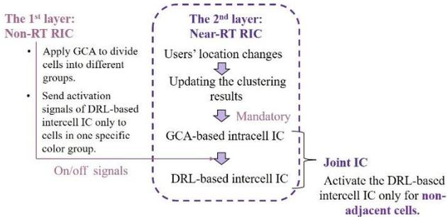
**Fig.2.** The framework of 2-layer joint IC.
