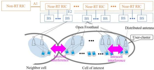
**Fig. 1.** Cellular system with cluster-wise distributed MU-MIMO under O-RAN architecture.
