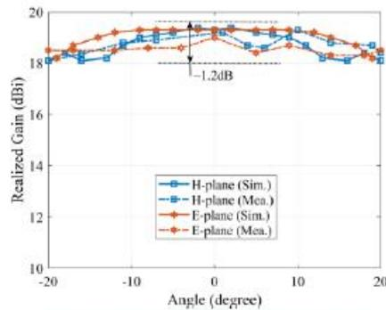
Good gain stability of lens with **less than 1.2dB variation**
