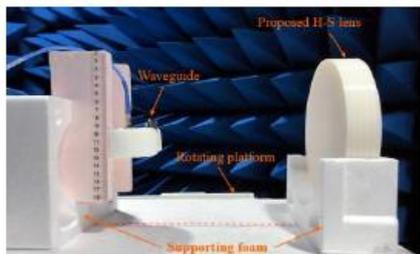
The waveguide placed at off-center position of lens leads to a steered beam
