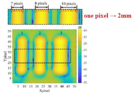
A spatial imaging **resolution of  $\sim 0.5\lambda$  ( $\sim 15\text{mm}$ )** is achievable with this measurement setup.
